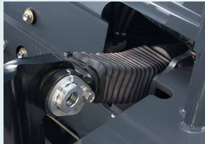
Tilt Cylinder Boots Each boot covers the exposed portion of the rod for the tilt cylinder, protecting it and the oil seals.
