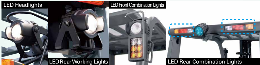
LED Headlights OPT LED Front Combination Lights OPT LED Rear Working Lights OPT LED Rear Combination Lights OPT Power-saving, long-life LED lights are available for the headlights and rear working lights.
